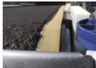
Separated particles transported to top of belt and drained to high dry matter content
